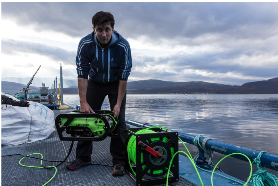
Figure 12 The Nofima ROV which is similar to those used in commercial salmon farming operations and which could be used to complete fast and relatively cheap urchin biomass surveys.
