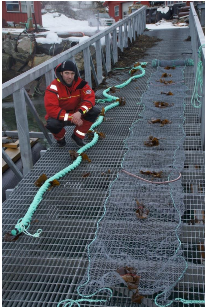
Figure 2 The weighted rope (Rope) and mesh panel (Panels) traps tested in the Experimental trap trials.
